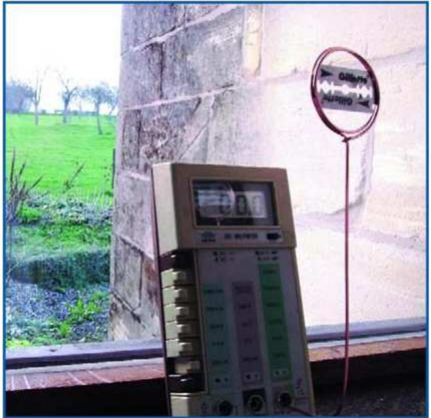
When you place this impressive looking apparatus looking apparatus on a windowsill during a thunderstorm and set the meter to the 200 mV range, you will, with a bit of luck, see nice deflections during lightning strikes. A nice thing is that you will see a build-up of static charge long before the flash, and immediately after the lightning flash the charge is gone.
