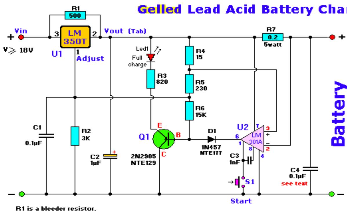
All resistors are carbon, 1/4 watt, 5% tolerance, unless otherwise indicated.
