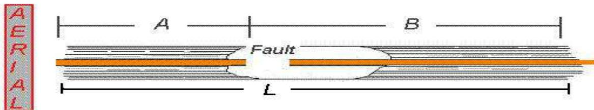
Measure capacitance of length A  $A = 350\text{pF}$
