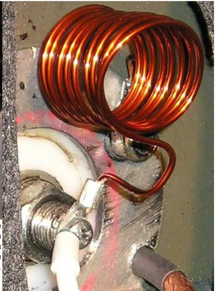
Properly matching the antenna impedance to the line impedance is important, especially if you're using an automatic antenna controller. And, if your HF antenna doesn't require matching to provide a low SWR then you need a better antenna, a better mounting position, or both!
