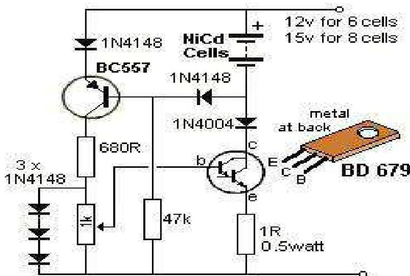
This NiCd battery charger can charge up to 8 NiCd cells connected in series. This number can be increased if the power supply is increased by 1.65v for each additional cell. If the BD679 is mounted on a good heatsink, the input voltage can be increased to a maximum of 25v. The circuit does not discharge the battery if the charger is disconnected from the power supply.
