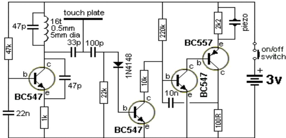
This circuit can be used to detect when someone touches the handle of a door. A loop of bare wire is connected to the point "touch plate" and the project is hung on the door-knob. Anyone touching the metal door-knob will kill the pulses going to the second transistor and it will turn off. This will activate the "high-gain" amplifier/oscillator.
