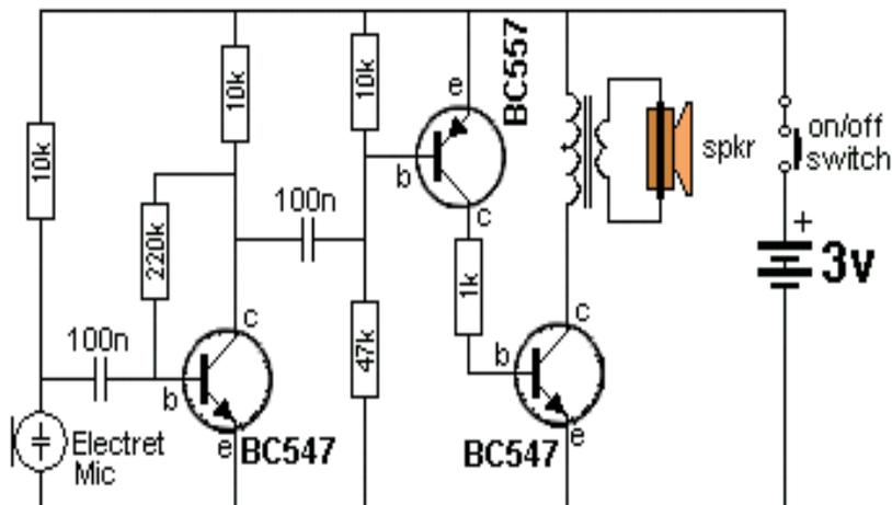
This circuit is a very sensitive 3-transistor amplifier using a speaker transformer. The biasing of the middle transistor is set for 3v supply. The second and third transistors are not turned on during idle conditions and the quiescent current is just 5mA. The project is ideal for listening to conversations or TV etc in another room with long leads connecting the microphone to the amplifier.
