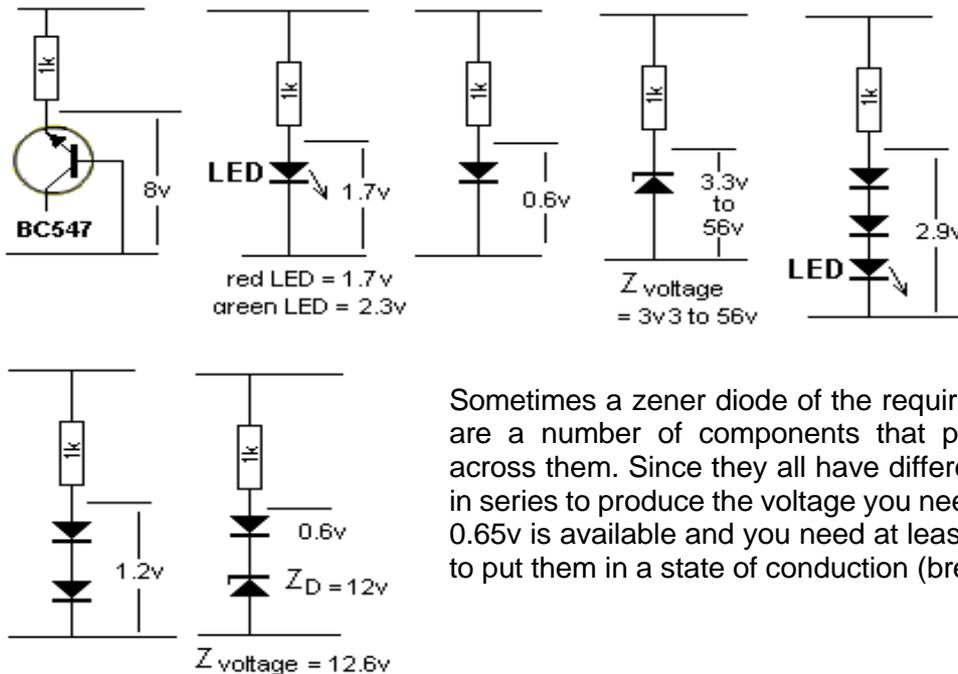
Sometimes a zener diode of the required voltage is not available. Here are a number of components that produce a characteristic voltage across them. Since they all have different voltages, they can be placed in series to produce the voltage you need. A reference voltage as low as 0.65v is available and you need at least 1 to 3mA through the device(s) to put them in a state of conduction (breakdown).
