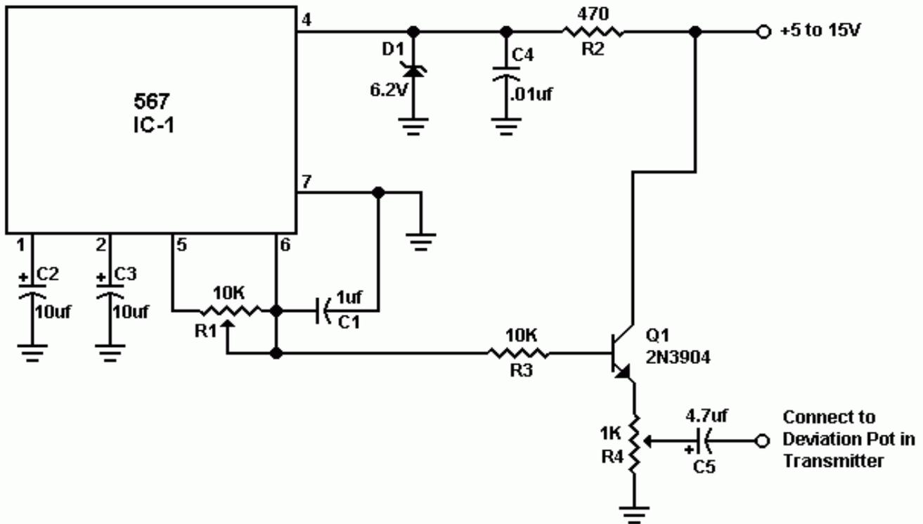
This easy circuit that can be constructed with mostly easily available parts on any general purpose circuit board. The only rigid requirement is that capacitor C1 be stable over a wide temperature range. Use only Mylar, Polyester or Metal film for capacitor C1. The frequency is determined by the following formula:
