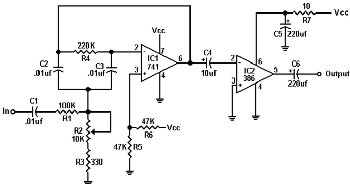
The circuit is a variable bandwidth CW filter using two IC's. The first IC is a 741 op amp used as an active filter and the second IC is a 386 audio amp IC. This circuit connects to the headphone or speaker jack of your HF rig. The volume is controlled by the volume control of your rig and R2 controls the bandwidth. There is plenty of audio to drive a small speaker or a pair of headphones.
