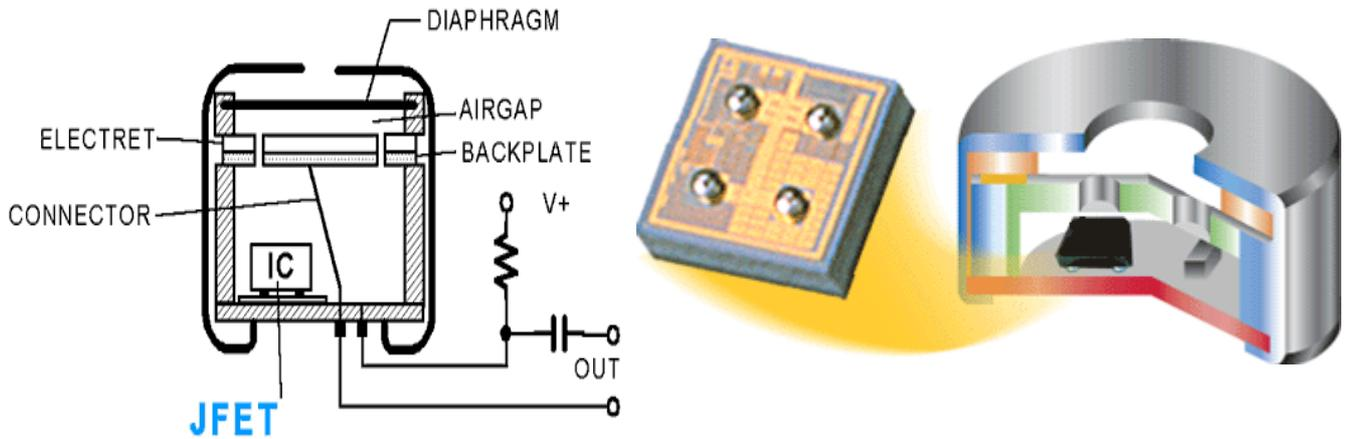
Electret Condenser Microphones (ECM) are used in almost every consumer and communication audio application. The total yearly volume of all ECM's is well over one billion units. Over the years, innovation in ECM's has concentrated mainly on lower cost production and smaller sizes. Other improvements of sensitivity, Signal-to-Noise Ratio (SNR), linearity, and supply current have not been addressed.
