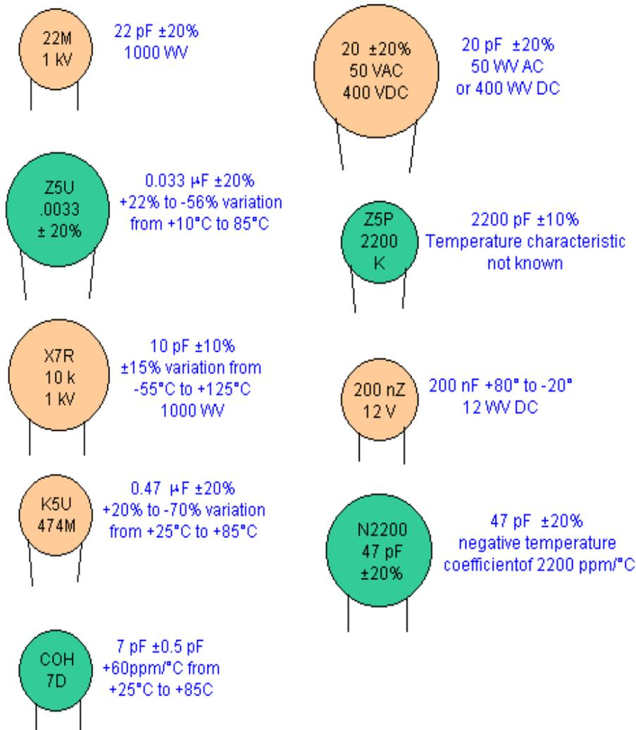
Ceramic disk capacitors have many marking schemes. Capacitance, tolerance, working voltage and temperature coefficient may be found. Capacitance values are given as number without any identification as to units. (uF, nF, pF) Whole numbers usually indicate pF and decimal numbers such as 0.1 or 0.47 are microfarads. Odd looking numbers such as 473 is the previously explained system and means 47 nF.
