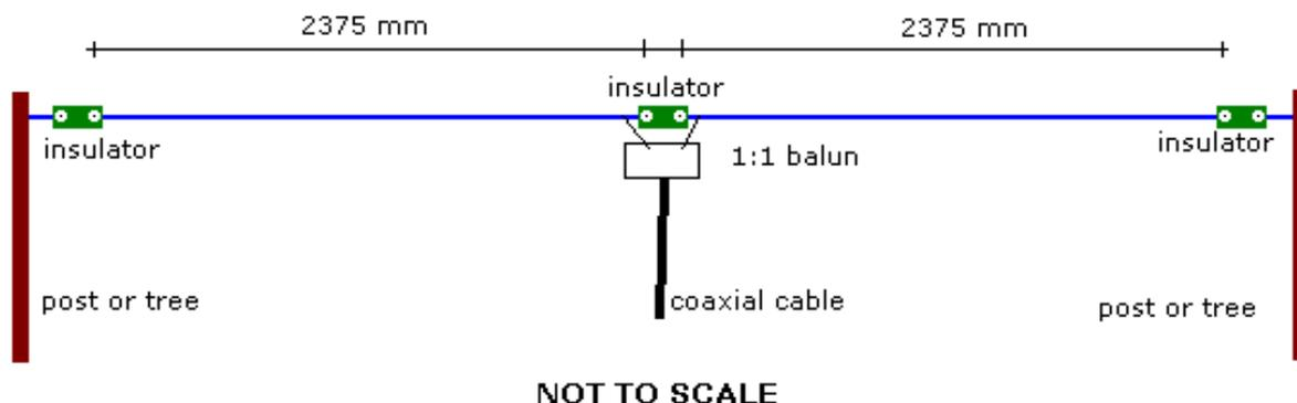
This particular antenna was dimensioned for use at 30 Mhz. You will note that the left and right hand halves are merely quarter wave sections determined by the formula given earlier. The input impedance (affected by many factors) is nominally 50 ohms.
