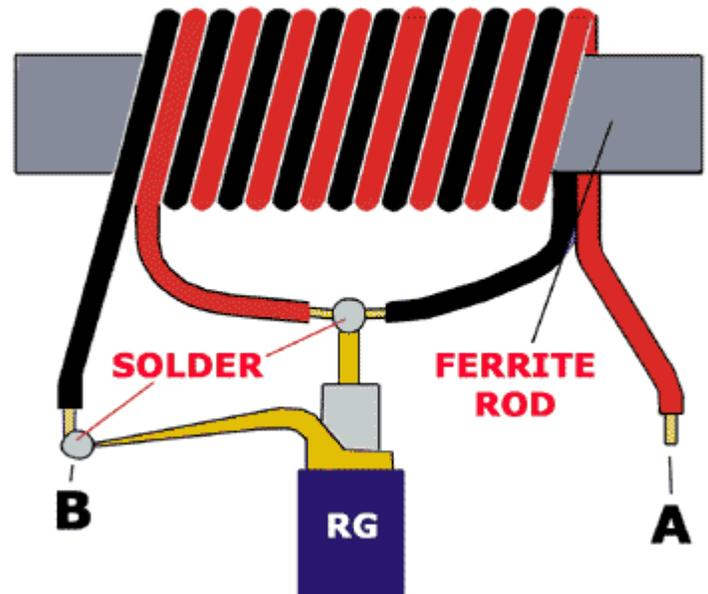
One or two ferrite rods are necessary for the Balun, depending on output power of your transmitter. The wire is a simple electrical-wire 1 - 1,5 mm (Double "Red-Black" wire for Loud Speakers) 9-10 turns on ferrite rod is enough but keep in mind before winding: "cut" the two cables (red & black in the picture above) of equal length.
