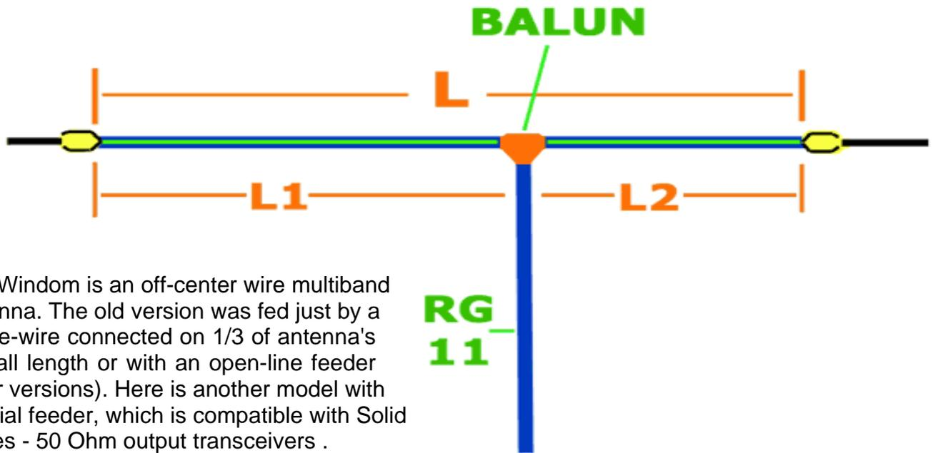
The Windom is an off-center wire multiband Antenna. The old version was fed just by a single-wire connected on 1/3 of antenna's overall length or with an open-line feeder (later versions). Here is another model with coaxial feeder, which is compatible with Solid States - 50 Ohm output transceivers .
