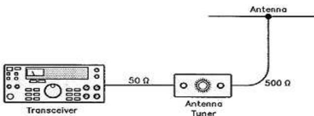
Most antenna tuners have an inductance rotary switch and two capacitors. The capacitors are often labeled ANTENNA and TRANSMITTER. In some antenna tuners the inductance switch is replaced with a continuously variable inductance, popularly known as a roller inductor.
