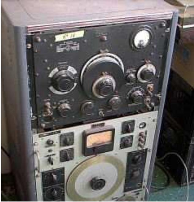
A . a General Radio Co of Cambridge USA a STANDARD SIGNAL GENERATOR SERIAL NO 307 TYPE 1001-A covering Frequency in - Kilo cycles & Megacycles top unit in photo.
