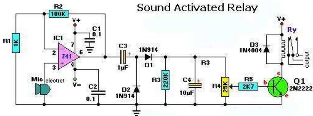
This relay remains dormant until the op-amp activates upon sound via the electret-microphone.
