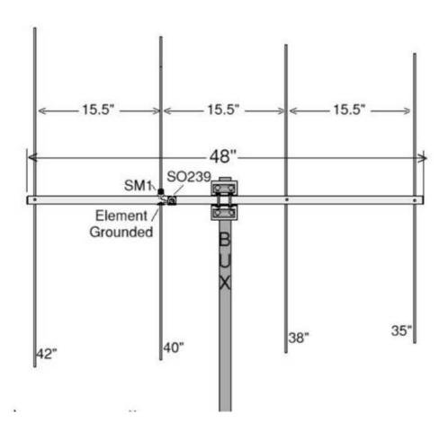
Four element, two meter beam, elements can be tubular aluminium or solid aluminium. This beam may be installed vertical, or horizontal. For optimum performance and gain, feed with 4:1 balun
