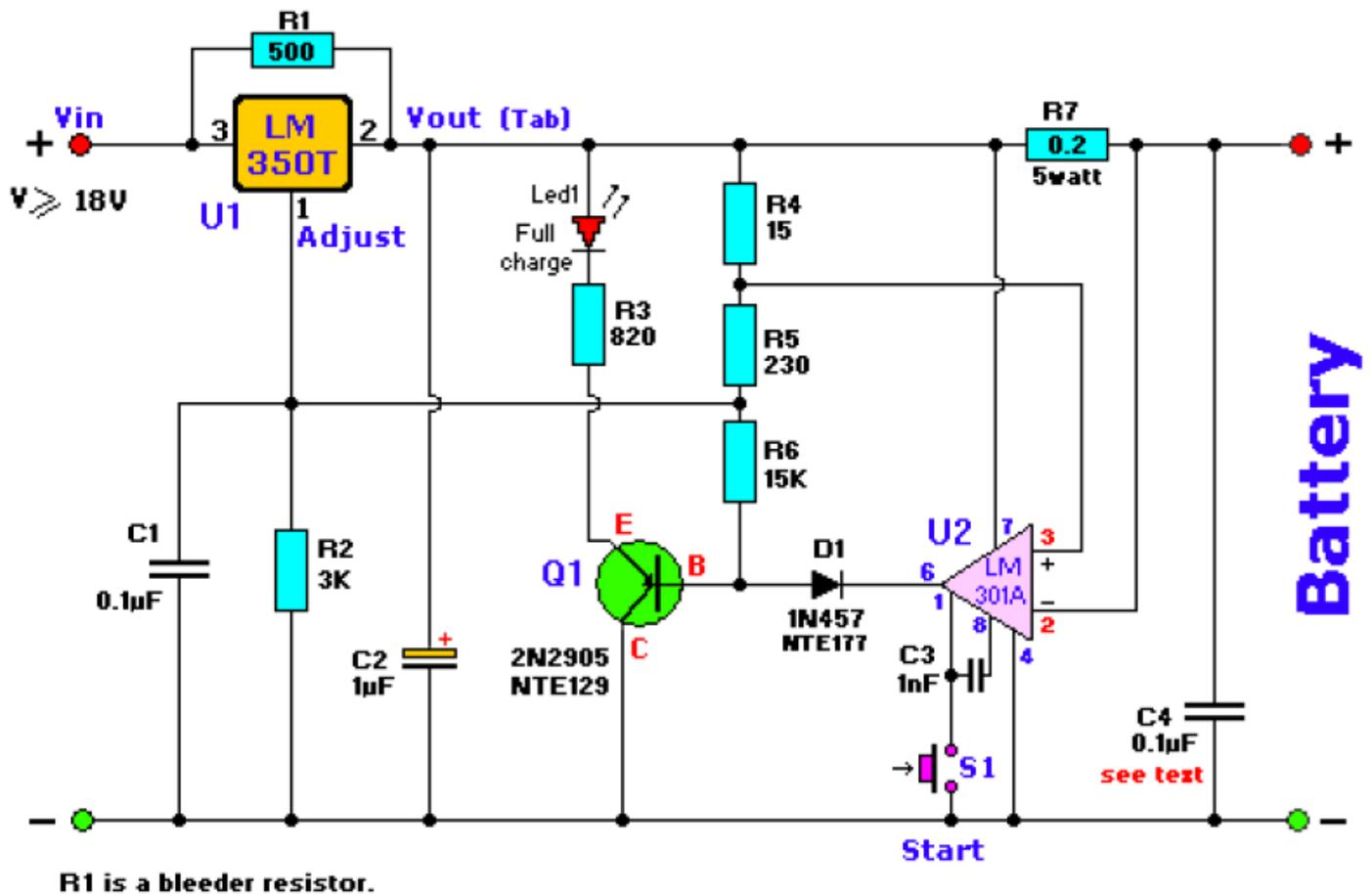
All resistors are carbon, 1/4 watt, 5% tolerance, unless otherwise indicated.
