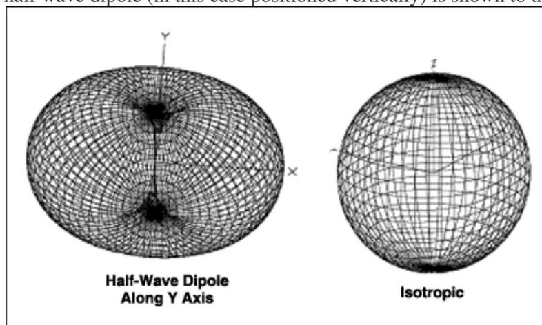
The donut-shaped radiation pattern of the dipole is totally different from the isotropic, i.e. in each direction we have a different amount of energy that is being radiated. This makes
