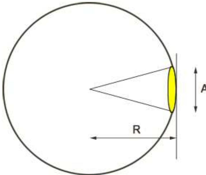
The higher the gain of the antenna, the smaller the aperture will be. In physics we get nothing for nothing; the gain of the antenna is in fact nothing but the antenna's ability to "concentrate" the radiated energy on one spot, just like a lens can focus a beam of light: the smaller the spot, the brighter the light.
