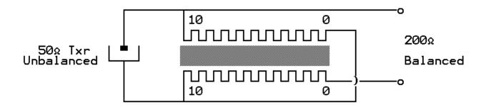
10 bifilar turns on a Amidon T 200-2 TOROID CORE. Make sure they are in phase & connected correctly.
